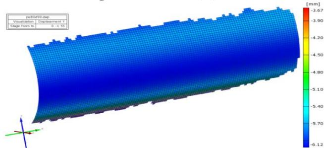
Fig.23. Displacement of the pipe in vertical direction ( $O_y$ ) [mm]
