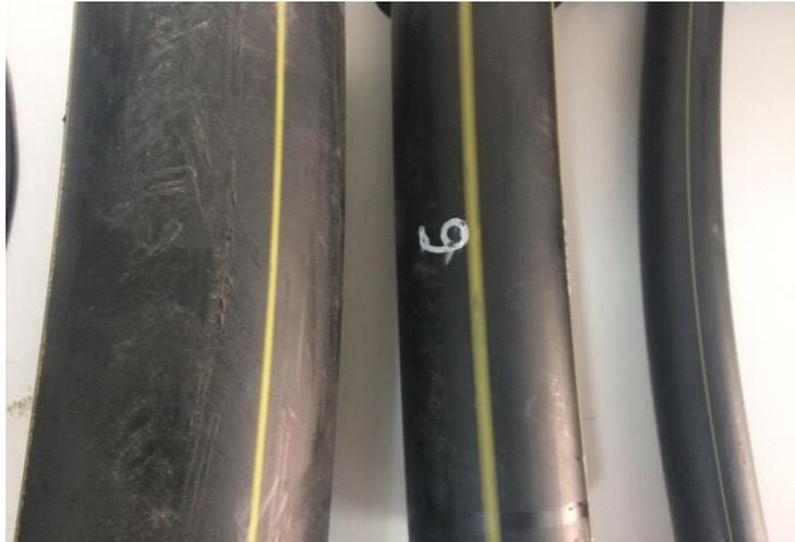
Fig.17. The specimens used for the testing are Dn 32, 63 and 90 mm in diameter
