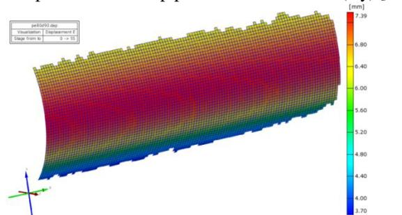
Fig.25. Total displacement of the pipe [mm]
