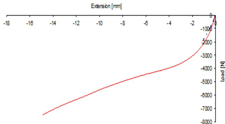
**Fig.21.** Experimental force-deformation characteristic curves for  $\Phi$  63 x 5.8 pipe
