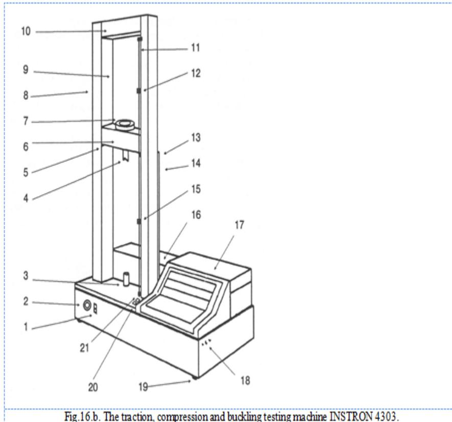
Fig.16 b. The traction, compression and buckling testing machine INSTRON 4303.
