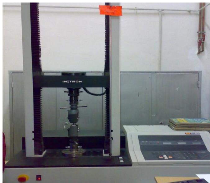
**Fig.16.a.** The traction, compression and buckling testing machine Instron 4303.
